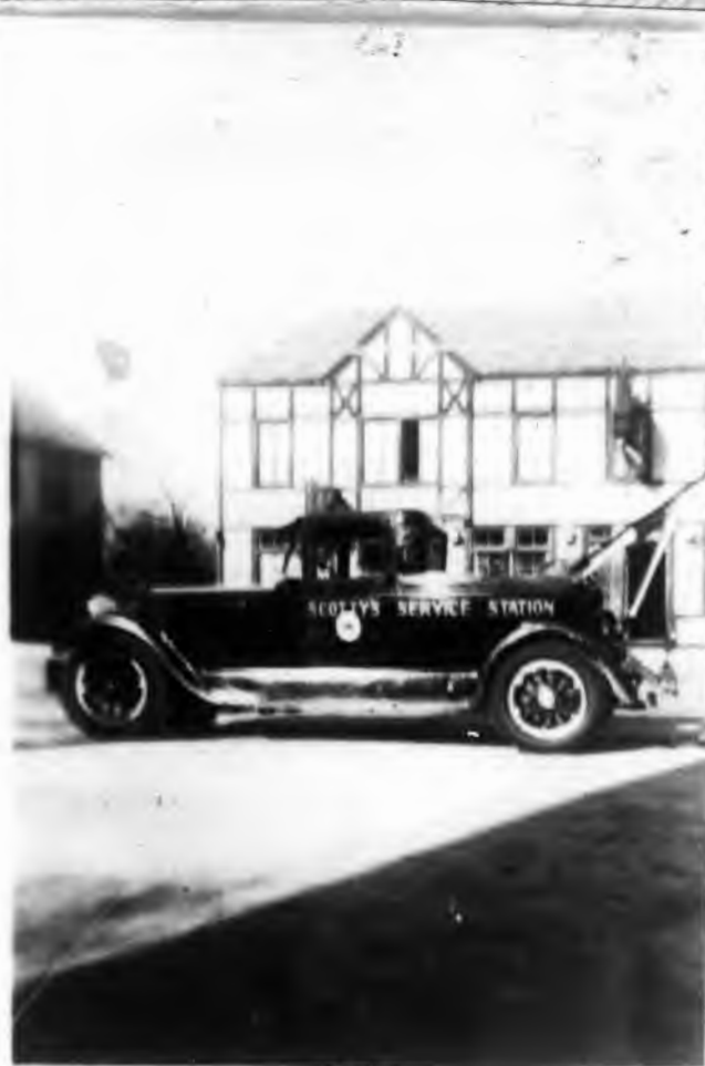
1930 Lincoln Sedan converted to hand-operated tow truck
